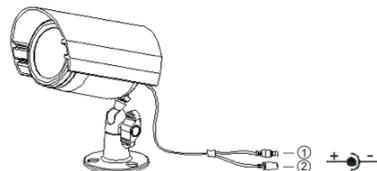
**NOTE:** Please use the correct power adaptor, DC12V (regulated), to operate this unit. The tolerance of this unit is DC12V ± 10%. Over the maximum DC12V power input will damage the video output connector (VIDEO OUT).
