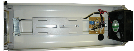
Shown above with optional 24 vac Heater and Blower Kit.
