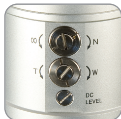
External Lens Adjustment Screws.
