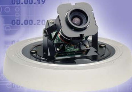
Inside of Dome
